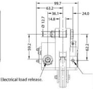
Emergency release cable connection point (5/16-24-2B UNF)
