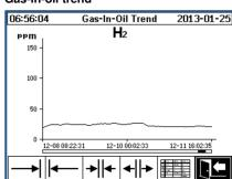
A graph displaying the trend over the time, in this case Hydrogen  $(H_2)$ , is shown.
