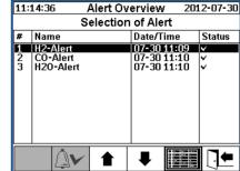
Display of alarm list. Details of each alarm and individual settings is shown.
