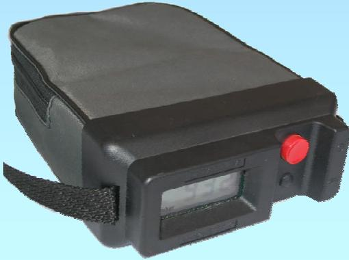
The manometer's prime function is to take accurate pressure readings of air filled telephone cables, but can also be used on other applications using non-corrosive gases. Based on a piezo-resistive sensor complete with its own laser trimmed temperature compensation, this manometer brings the user new excellence in pressure monitoring. With only two controls on the front escutcheon, the operation of the manometer is simple, quick and requires no setting time.
